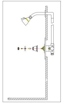
Install valve (G1), making sure 'up' outlet is facing up.
