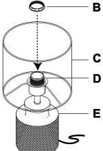
SECURE THE LAMPSHADE (C) BY TURNING THE SOCKET RING (B) ONTO THE SOCKET (D)
