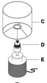
PLACE THE LAMPSHADE (C) INTO BASE (E) BY PUTTING METAL WASHER OF SHADE (C) ON THE SOCKET (D).
