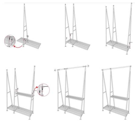
Step 5: Now insert Short Metal Rod (F) on the top of the Panels from threaded bore as per shown in illustration. Then, insert Large Metal Rod (G) such that its large threaded bore fit into end of Metal Rod (F) rotate rod clockwise until tight and then insert Knob(H) on the both end and rotate clockwise until tight.
