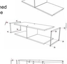
secure a screw at this mark directly into the wall and stud when instructed to do so below. Do not use a provided anchor at this stud location because the anchor cannot penetrate wood.
