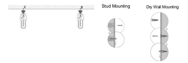
With the help of another person, hang the item to the wall so that the D-ring engage screw heads.
