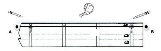
Connect the two points (A, B) with a light pencil line. Use a level to ensure that the line is level.
