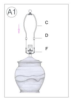
Raise the Harp Caps (D) and insert the bottom ends of Harp (C) into the Saddle (F)
