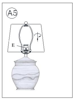
Insert the specified light bulb into the Socket (E). DO NOT EXCEED THE SPECIFIED WATTAGE.
