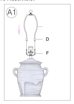
Raise the Harp Caps (D) and insert the bottom ends of Harp (C) into the Saddle (F)
