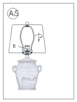
Insert the specified light bulb into the Socket (E). DO NOT EXCEED THE SPECIFIED WATTAGE.
