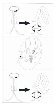
6. Connect the NEUTRAL FIXTURE WIRE to the NEUTRAL JUNCTION BOX WIRE (usually white insulation). Fasten each together with a Plastic Wire Nut Connector (A) by twisting the connector in a clockwise direction and wrap the connection with electrical tape. Be sure that no wire strands are exposed.
