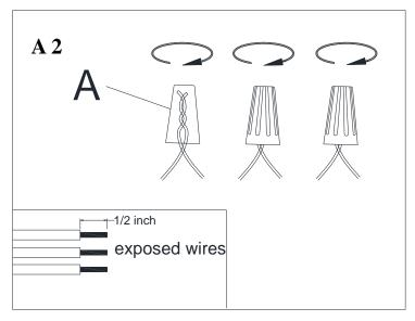
7. Connect the HOT FIXTURE WIRE to the HOT JUNCTION BOX WIRE (usually black insulation). Fasten each together with a Plastic Wire Nut Connector (A) by twisting the connector in a clockwise direction and wrap the connection with electrical tape. Be sure that no wire strands are exposed. **DO NOT REVERSE THE HOT AND**
