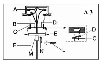
11. Insert the 2 Canopy Screws (E) through the Canopy (F) and into the threaded holes of Crossbar (D), tighten each with a screwdriver until secure.
