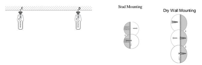
With the help of another person, hang the item to the wall so that the D-ring engage the screw heads.
