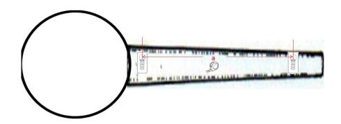
With the back of each Bread Paddle facing away from the wall, hold it against the wall at a desired mounting location. Mark two reference points(A, B) on the wall as shown
