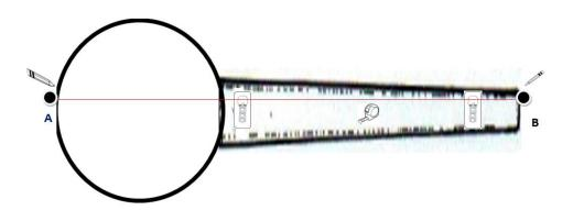
Connect the two points (A, B) with a light pencil line. Use a level to ensure that the line is level.
