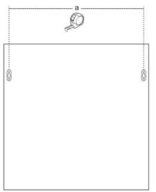
With the back of the item facing away from the wall, hold it against the wall at a desired mounting location. Mark two reference points (A, B) on the wall as shown.
