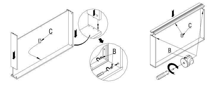
6. Turn the cam locks (B) clock-wise with a Phillips head screwdriver (approx. 210°).
