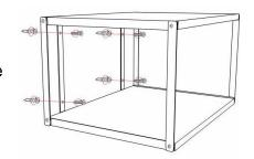
With the help of another person, hold the item upright and against the wall so that the four through holes align with either a stud-aligned mark or an installed anchor. Use a screwdriver to secure a provided screw through each through hole and into the wall or an
