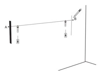
3 Connect the two points (A, B) with a light pencil line. Use a level to ensure that the line is level.
