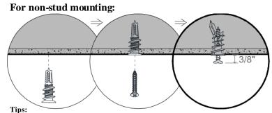
The anchor is self-drillable. No pilot hole required.
