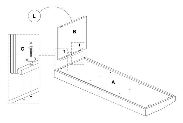
2. Attach the Dividers (C) on the Top (A) by aligning wood dowels and pre-drilled holes. Secure by Screw (G) using a Phillip head screwdriver.
