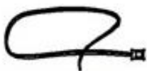
Nylon Strap (2) To hold article tying with plastic bracket and metal security hanger.
