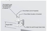
Step 4: To prevent any wood from splitting when screws are secure therein, we recommend that pilot holes be drilled at the marked locations for the brackets.
